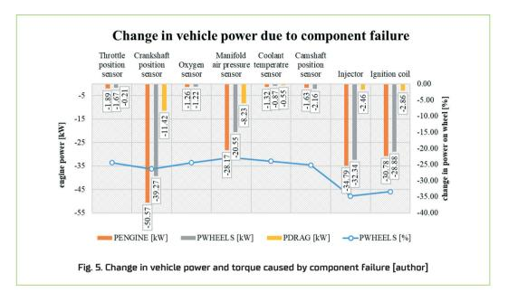
The graph (Figure 5) shows the reduction in performance due to disconnection of a given component. Power loss is given in kW. The power loss to the wheels, the engine power loss and the magnitude of the power loss are determined.
